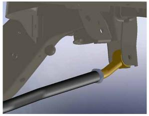
Mount Chassis End (A) of adjustable trackbar to the chassis bracket by loosely installing the original mounting hardware.
