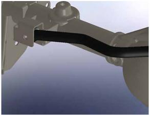
O <u>Loosely</u> install the original mounting hardware.
